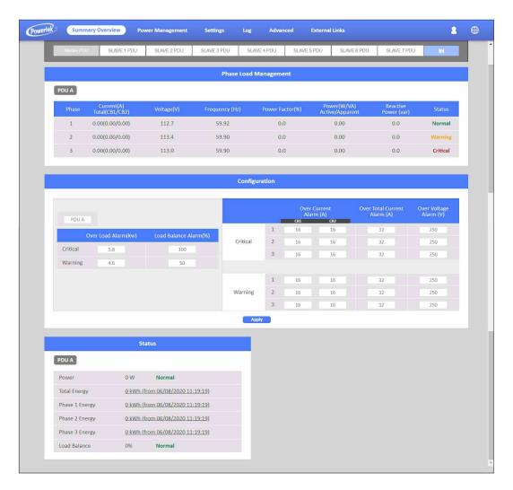
The POWERTEK PDU provides a graphic user interface that can be viewed from a web browser such as Internet Explorer. This enables users to access and control the device outlets and subsequently, its output devices remotely from users' desktop, laptop, PDA, or even users' mobile phones. This section provides instructions about how to use the web interface to configure and control the PDU remotely.
