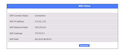
**Step 4:** Please access the Wi-Fi IP address (example IP: 172.31.1.33) from web browser and make sure the Wi-Fi dongle has workable.
